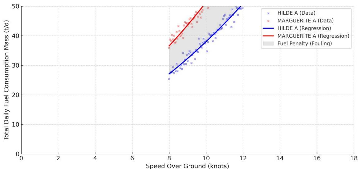
The regression chart does not show data between 0 and 8 knots because the data was intentionally generated starting from 8 knots due to scattered outliers (Jones, 2017), likely idle/port periods, or invalid voyage data.
